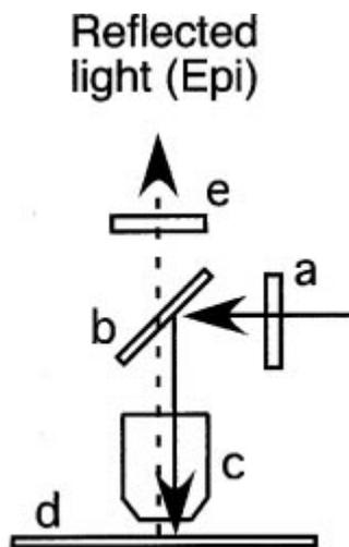
Fig.1. Schematic diagram of optical pathway of typical epifluorescence microscope. (a – excitation filter, b – dichromatic mirror, c – objective lens, d – specimen, e – emission filter)
